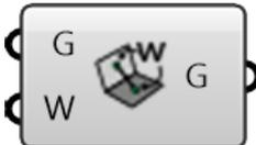
**Custom Node Weight (cNodeWeight)** assigns a set of custom values as weights for each of the nodes in a MeshGraph. The set of values is remapped to the 0...1 interval.
