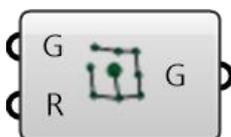
**Set Tree Root (TreeRoot)** This tool sets the root of a MeshGraph to an arbitrary node.
