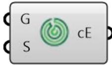
**Orange Peel Edges (OPE)** The tool creates a pattern of nodes that develop concentrically radiating from a set of mesh features. The features are defined by a tree of mesh vertex ids provided by the user. The vertex ids are grouped in branches each defining a feature that ripples its own “waves”. The component outputs the edge ids for the edges that span between the waves. This is useful in order to assign weight to those edges and thus facilitate a segmentation in concentric strips.
