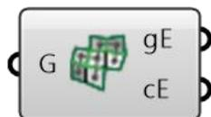
**Edge Types (eTypes)** This component extracts the edges from a base mesh by their MeshGraph statute. The edges can be either a graph edge (one connecting nodes inside the graph) or a cut edge (one that was deleted from the dual graph in the segmentation/tree making process)
