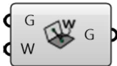
**Custom Edge Weight (cEdgeWeight)** This tool assigns a set of custom values as weights for each of the edges in a MeshGraph. The set of values is remapped to the 0...1 interval.
